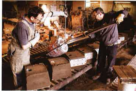
03 CASTING OF THE SIGNAGE BY SCHIAVELLO AT MULLHOLLAND FOUNDRY. PHOTOGRAPHY: SOREN LUCKINS.
