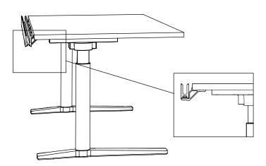
Suitable for fixed height or height adjustable bases, shown with Krossi single stage legs. The rail moves with the height adjustable worksurface.
