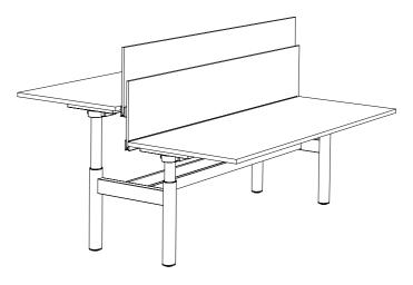
Two single sided rails fitted to height adjustable desks back to back.
