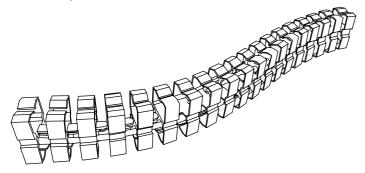
The flexible "articulation" provides the additional benefit of creating dynamic Krossi configurations. These configurations can be rapidly manipulated because the Cable Articulator can bend without structural compromise. The knuckle assembly is secured with pins which enable the dynamic Channel configurations. The Cable Articulator is made up of multiple modular components and is fixed to the Channel using a snap lock fastening which locks into the "Channel inner end cap."
