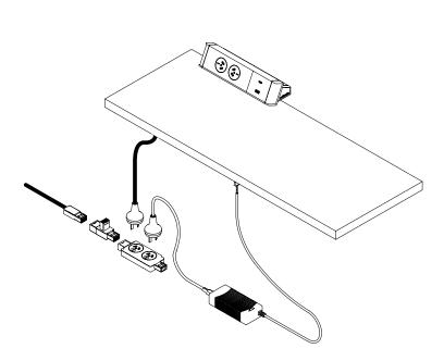
100W USB A-C in desk charger is connected via a three pin plug from the power supply, this is plugged into a GPO located below the desk in a cable tray or wire basket
