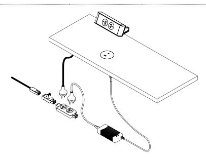
100W USB A-C in desk charger is connected via a three pin plug from the power supply, this is plugged into a GPO located below the desk in a cable tray or wire basket
