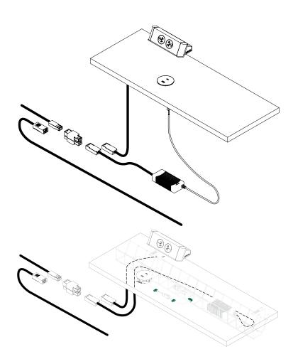
100W USB A-C in desk charger is connected via an installation lead from the power supply into a junction located below the desk in a cable tray or wire basket
