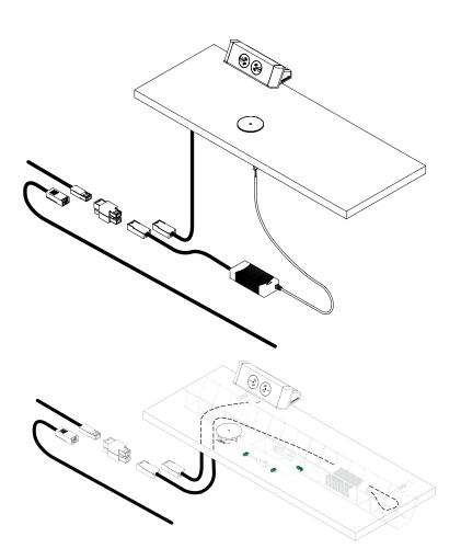
15W Qi charger is connected via a power supply this is plugged into a GPO socket located below the desk in a cable tray or wire basket
