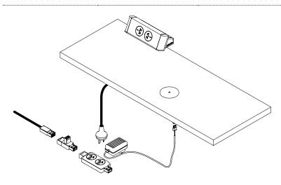
15W Qi charger is connected via a power supply, this is plugged into a GPO socket located below the desk in a cable tray or wire basket
