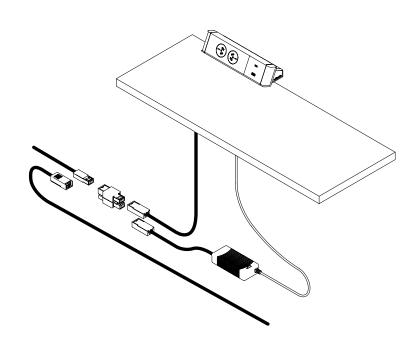
100W USB A-C in desk charger is connected via an installation lead from the power supply into a junction located below the desk in a cable tray or wire basket
