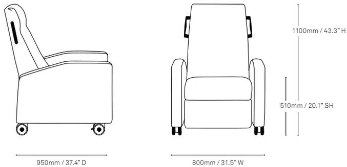
All measurements are in millimeters
